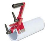
Recommended by plastic pipe manufacturers. Releasable grips. Counter-blade. Capacity: Ø 32 to 250 mm. Thickness: to 12 mm. Chamfering angle: 15° on plastic pipes. Pivoting counter-blade adjustment.
